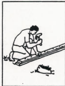
MAKE BEARERS USING TWO 6x2'S
