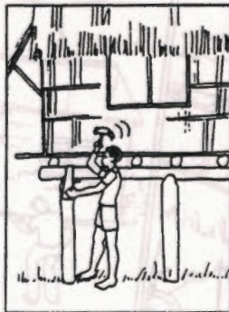
STRAP WOOD BEAMS TO FOUNDATION POSTS WITH METAL STRAPS.
