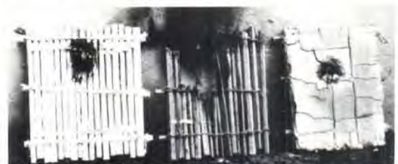
Stems being fire tested. Mud plaster or fire resistant paint reduce the risk of burning.
